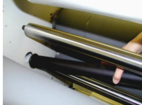
**Figure 16: Inserting Cooling Tube**
