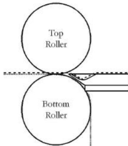
**Figure 18: Feeding Images under the print guide**
