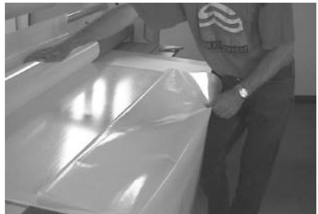
**Figure 24: Mounting decals onto substrates**
